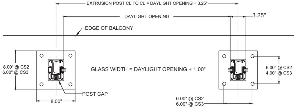
Note: Post to post spacing by engineering calculations. Max post spacing center to center is 5 feet.
