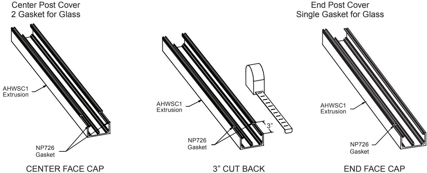
End Face Cap: Install gasket NP726 on the side of the post where glass will be installed only.
