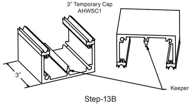
**IMPORTANT** – Temporarily hold glass in place with temporary cap at all four corners of glass. Align the keeper with plastic clips and push until cap locks in place. To remove temporary cap **SLIDE CAP UP OR DOWN** until it disengages from the plastic clip. Avoid pulling the cap horizontally. If clips are damaged in this process, replace with new ones.
