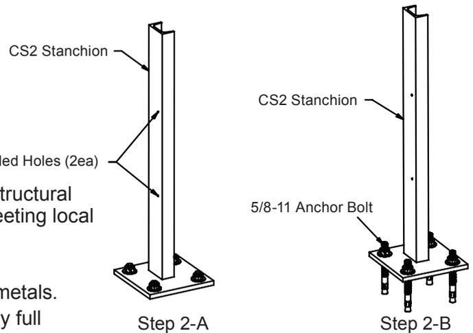
Securely fasten each stanchion with (4) 5/8" diameter structural anchor bolts as specified by structural engineer and meeting local building code.
