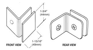
**NOTE:** The Clamps shown on this page can also be used in a glass-to-glass application. For information on this see pages 4T-9 and 4T-10.
