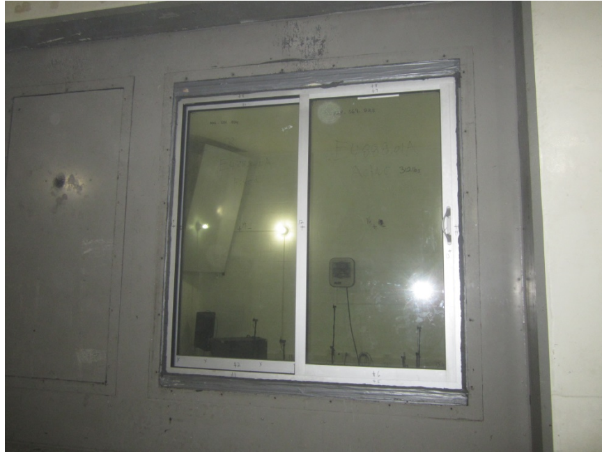
Receive Room View of an Installed Test Specimen
