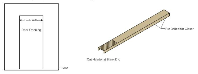
2. Drill Jig for 4" Header on Side 1, and Drill Jig for 4-1/2 Header on Side 2.
