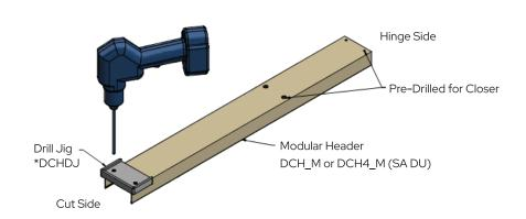
For shear block anchorage hole preparation, secure the Drill Jig firmly to the blank top side of the header. Use a 0.203" drill bit. Hold the jig steady from the side to maintain stability during drilling.
