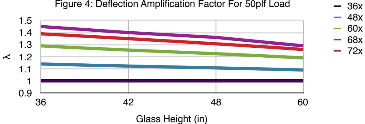
Figure 4: Deflection Amplification Factor For Wind Load
