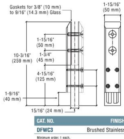
Clamp anchorage strength is same as calculated for the AFCW3 clamp.
