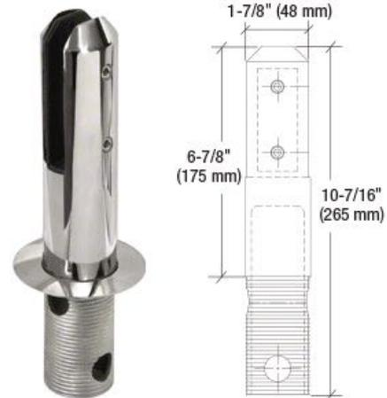
Moment is resisted by pry out from concrete. The grooves on the end of the rod prevent withdrawal.
