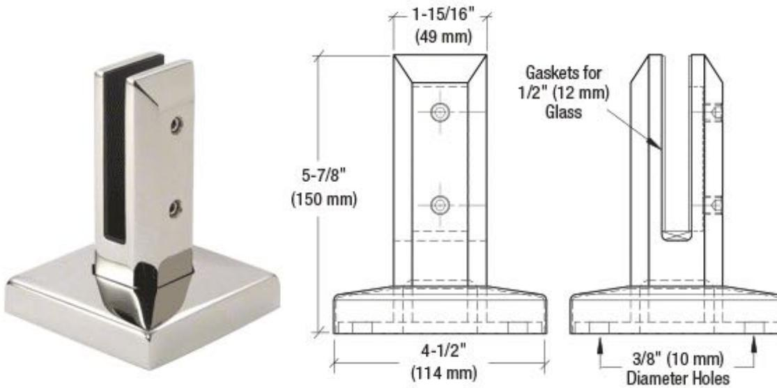
One piece stainless steel clamp with base shoe for surface mounting. Glass is locked into clamp by tightening two set screws which press a bearing plate against the glass.
