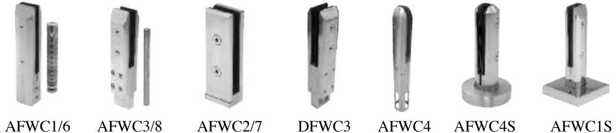
The Friction Fit Clamps are intended for installations without holes through the glass. These clamps don't have a through glass bolting option and are intended for locations with lesser wind loads or small light sizes and where fall protection typically isn't required.
