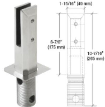
Anchorage is achieved by embedding clamp base into hole in concrete and grouted in place.
