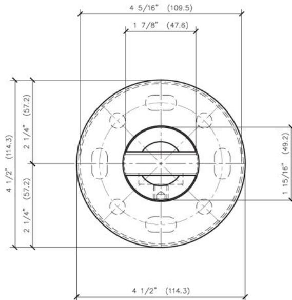
**BASE PLATE MOUNTED TO CONCRETE -**
