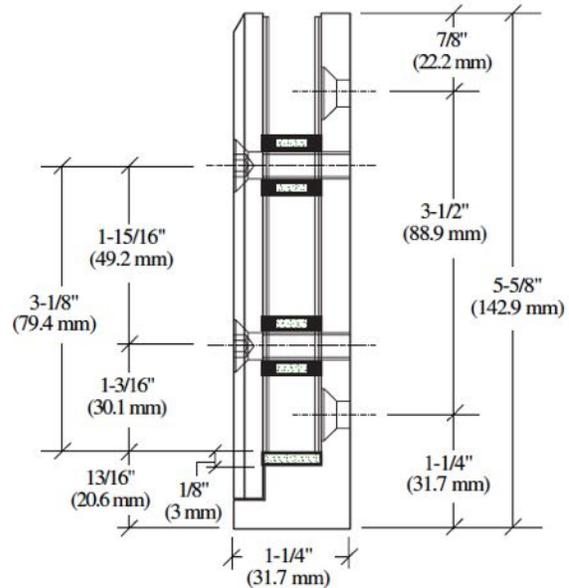
For anchorage to concrete using two 1/4" x 2-1/2" Tapcon screws with 1.75" effective embedment:
