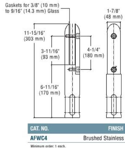
Clamp must be installed with bolt through the glass.
