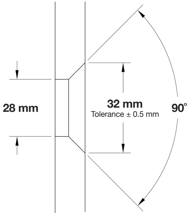
Drill a 28 mm diameter hole through the glass. Using the BDC112, countersink the glass to the approximate width shown. The exact depth of countersink should be determined by test fitting the CAPF1420 on a test piece of glass before production begins. Occasional random sampling of holes should be done to assure consistent fabrication.
