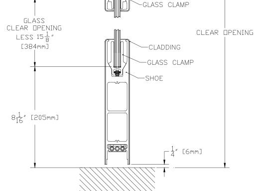
6" SQUARE DOOR RAIL TOP CLAD 10" SQUARE DOOR RAIL BOTTOM CLAD WITH CLAD HEADER
