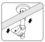
Loosen clamp to install sliding tube.
