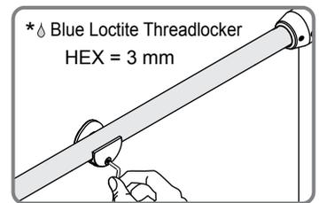
\* Blue Loctite Threadlocker is recommended on all screw threads during final assembly.
