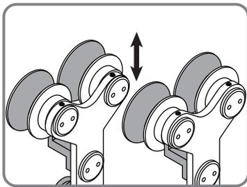
Loosen Top Rollers so they easily move up and down.
