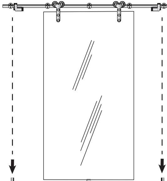
Install Floor Stops below Left and Right Door Stops. Rubber side faces door.
