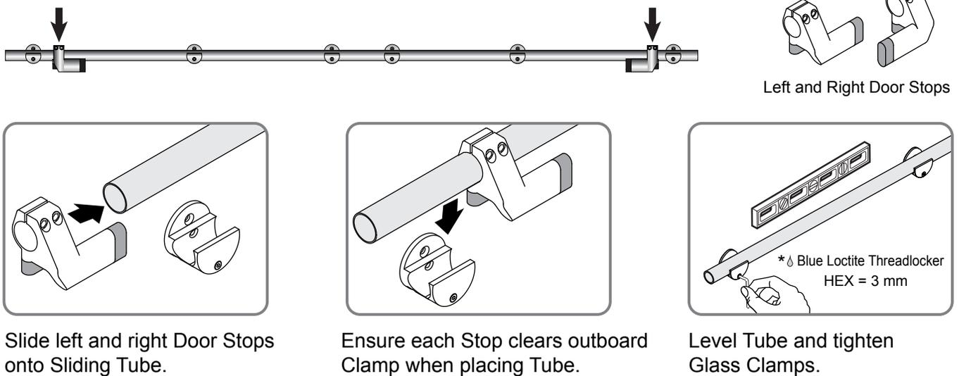
\* Blue Loctite Threadlocker is recommended on all screw threads during final assembly.
