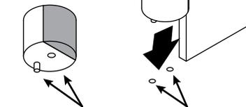
Floor Stop anchored at one end. Drill holes for screw and anchor to install.
