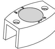
Position Floor Guide to align with wall.
