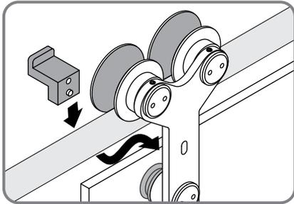
Fit Anti-Lift Block under Sliding Tube.
