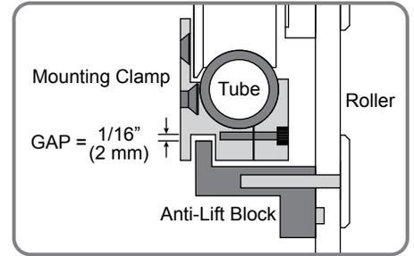
Adjust Anti-Lift Block so Rollers move freely through Mounting Clamps.
