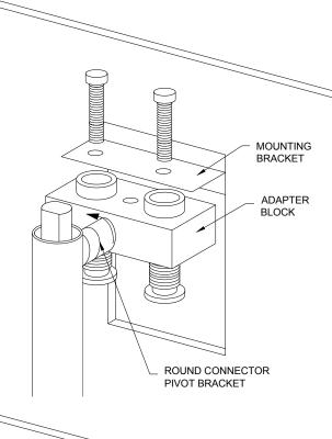
2.A. FOR GLASS MOUNT HANDLE. Remove Socket Head Cap Screw from Interior Pivot Bracket and Exterior Bracket. Be careful not to lose Gaskets located between Interior and Exterior Brackets. →
