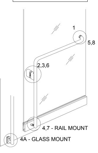
1. Install stud with locking nut through washer w/gasket and hand tighten.
