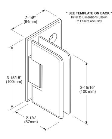
Wall Mount Hinge - Offset Back Plate (5° Preset Pivot Pin) CAT NO. COL544
