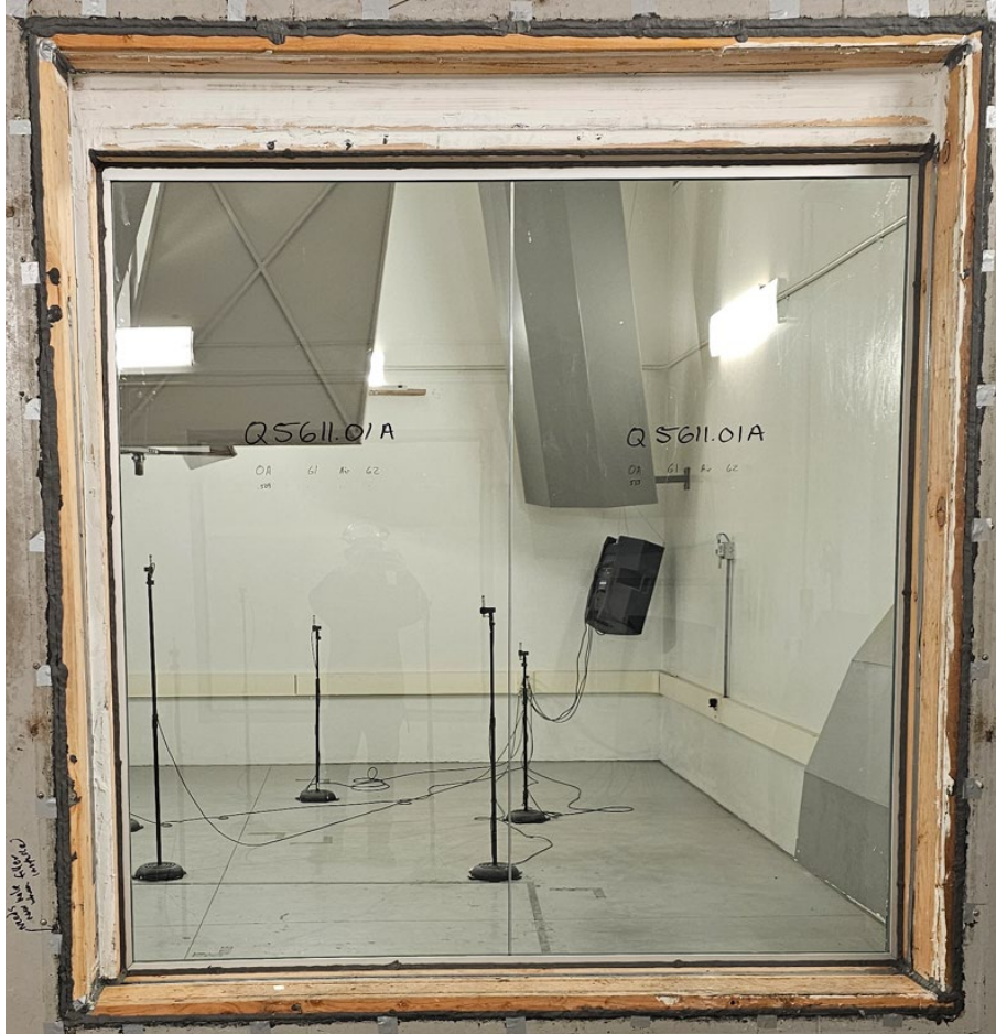
Photo No. 2 Source Room View of Installed Test Specimen
