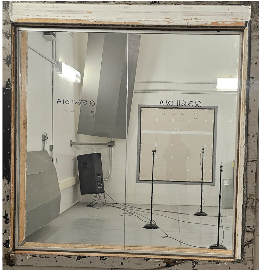
Photo No. 1 Receive Room View of Installed Test Specimen
