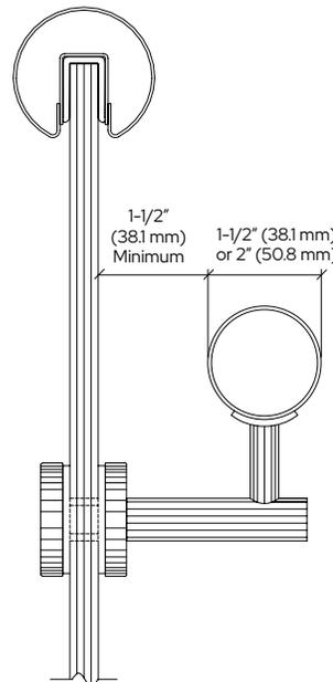
The hand grip portion of the Hand Rails shall not be less than 1-1/4" (31.7 mm), and no more than 2" (50.8 mm) in cross sectional dimension.
