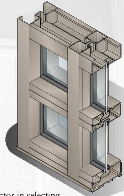
Fabrication and installation labor costs have always been a decisive factor in selecting framing systems for storefront projects. United States Aluminum offers cost efficient versatile Center Glazed Systems with clean lines and superb performance. All series may be interior or exterior glazed. A top load E.P.D.M. gasket is used to position and weatherseal the glass in the aluminum pocket. Center Glazed Systems are compatible with most United States Aluminum Entrance Doors.
