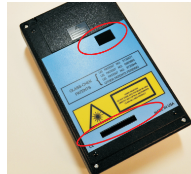
Above: Back of GC3200 meter with the two lenses circled. Use clean compressed air to clean the lenses.
