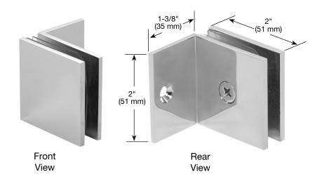
Material: Solid brass Glass Thickness Range: 3/8" (10) to 1/2" (12 mm) thick glass Hole Size Required: 5/8" (16 mm)
