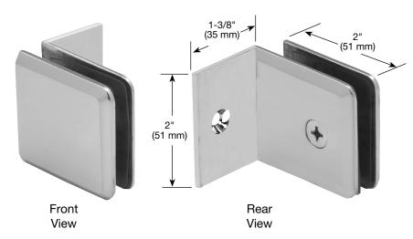
Material: Solid brass Glass Thickness Range: 3/8" (10) to 1/2" (12 mm) thick glass Hole Size Required: 5/8" (16 mm) or 3/4" (19 mm) diameter
