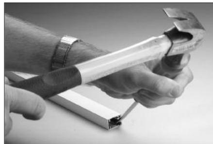
Diagram 8 - Crimping Weatherstrip Channel
