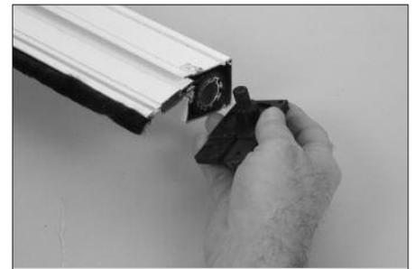
Diagram 3 - Installing End Cap
