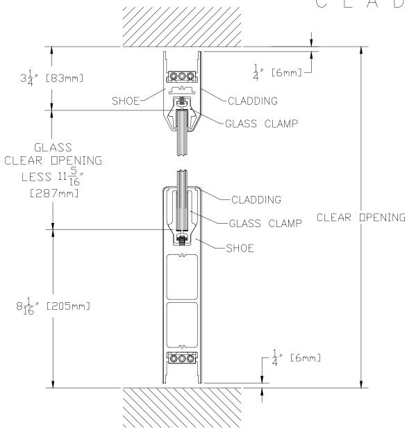
4" TAPERED DOOR RAIL TOP. CLAD OR NON CLAD 10" SQUARE DOOR RAIL BOTTOM. CLAD ONLY
