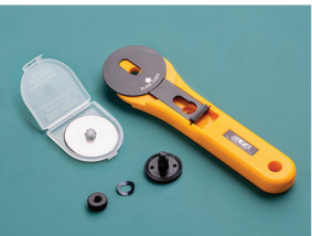
Pull the handle off of the stem that holds the blade and set it to the side.
