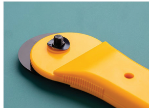
Place the washer back onto the stem with the curve facing up like a bowl.
