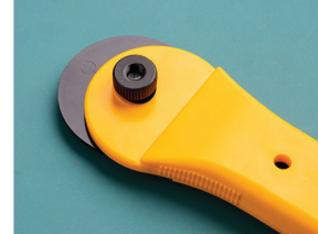
Next place the washer back onto the stem and tighten until the front disk begins to spin. Do not over tighten.
