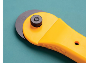
Next place the washer back onto the stem and tighten until the front disk begins to spin. Do not over tighten.
