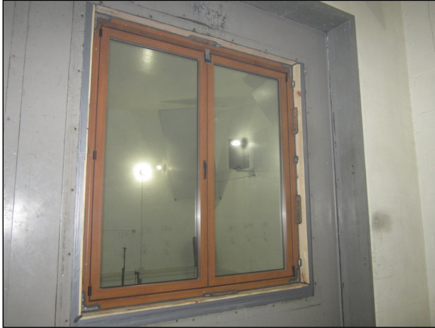
Receive Room View of Installed Specimen
