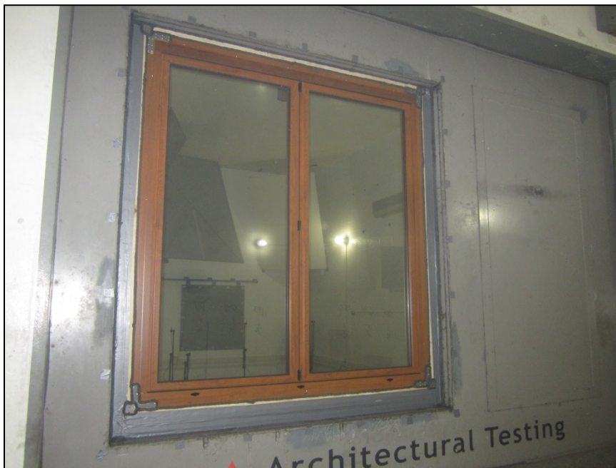
Source Room View of Installed Specimen
