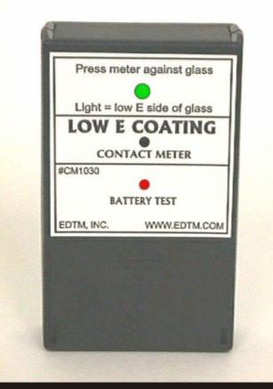
The CM1030 is a simple instrument that detects any conductive surface, including Low E coatings on single sheets of glass. The tester has 4 non-scratch pads on the back-side of the meter that allow you to test for conductive coatings. Simply press the meter against a piece of glass to determine if the surface you are touching contains any conductive (Low E) coatings.
