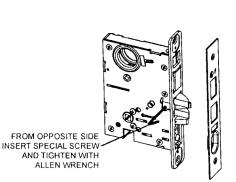
4. Reinstall the special screw and tighten securely with the provided allen wrench.
