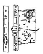
1. Remove special screw with provided allen wrench
