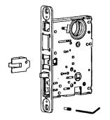
2. Pull latch bolt out of lock
