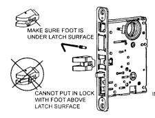
3. Rotate Latch bolt 180° and reinstall into lock, pushing the latch bolt into the lock and then releasing.
