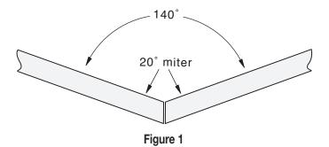
To determine the correct miter to use on each piece, use the following formula: **FORMULA: 180 minus "A" divided by 2 = your miter** "A" = angle
