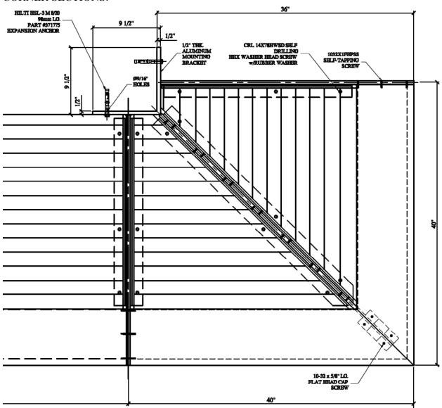
Strength of corner assembly: Corner bar tributary load: Triangular load: (0.33\*0.707)U at wall to (3.33\*0.707)U at end  $M = 0.233U*4.243'^2/2 + 2.35U*4.243^2/3 = 16.2U$  U = 3.5+u M = 56.7 + 16.2uBar and weld has same strength as previously checked and therefore will not control the allowable loads.
