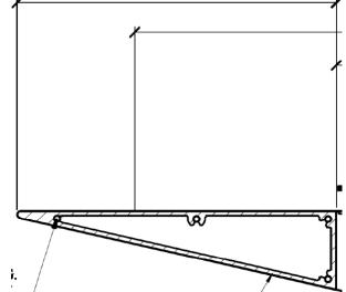
ATTACHEMENT TO WALL: Out rigger bar is welded to wall plate. Weld strength in accordance with ADM Section 7.
