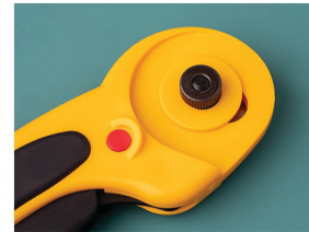
Next place the nut back onto the stem and tighten until the front disk begins to spin. Do not over tighten.
