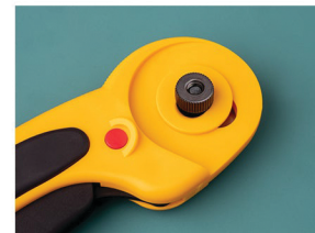
Next place the nut back onto the stem and tighten until the front disk begins to spin. Do not over tighten.
