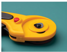
Place the plastic washer back onto the stem followed by the metal washer with the curve facing up like a bowl.
