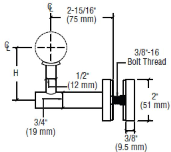
For strength of bracket on glass refer to HR2S calculations
