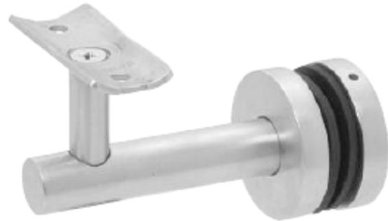
Mounting plates attached through glass with 3/8" threaded rod. Bracket strength will be determined by couple between threaded rod in tension and compression in mounting plates on glass.
