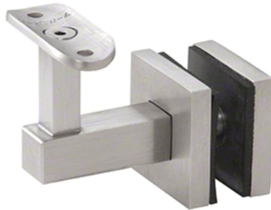
Mounting plates attached through glass with 3/8" threaded rod. Bracket strength will be determined by couple between threaded rod in tension and compression in mounting plates on glass.
