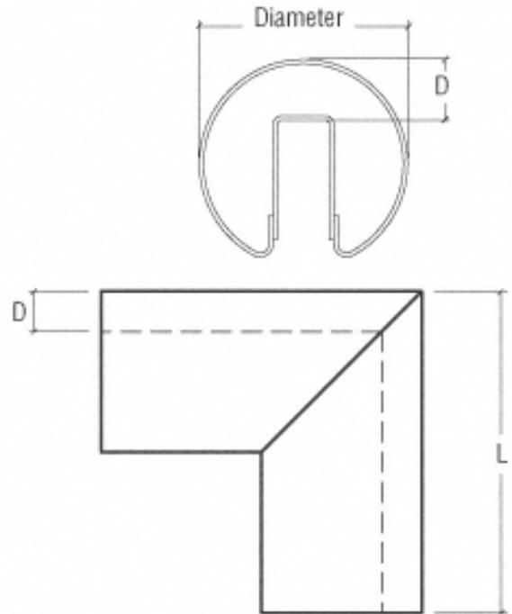
When the 6063-T6 aluminum alloy is welded the tempering is lost within the area of the weld affected zone reducing the allowable stress in the tubes to 5.5 ksi within 1” of the weld. This reduces bending strength to 30% of the bending strength for the unaffected cap rail.
