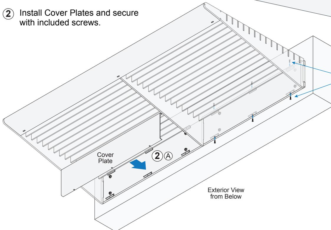
Secure at top and bottom holes with included #10-32 x 3/4" PFHMS.
