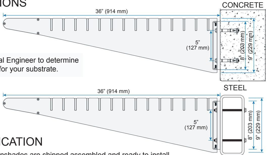
NOTE: Consult a Structural Engineer to determine the appropriate fasteners for your substrate.
