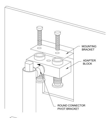
2.A. FOR GLASS MOUNT HANDLE. Remove Socket Head Cap Screw from Interior Pivot Bracket and Exterior Bracket. Be careful not to lose Gaskets located between Interior and Exterior Brackets. →
