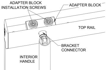
aligning top pivot bracket connector with the hole on the rail, please refer to the CRL Door Rails installation instructions for possible adjustments of the top rail.
