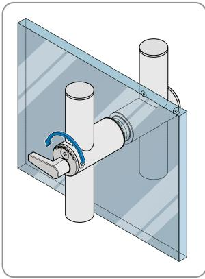
2. Remove the assembly bolt and the two lock housing screws that secure the thumb turn assembly in the lock housing, set these aside for later use during the installation of the Lock Indicator. Remove the thumb turn assembly.
