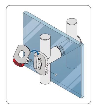
8. Secure the cover to the thumb turn using the two cover screws.
