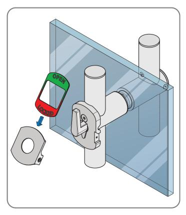
7. Work the assembly over the thumb turn and spacer washers.
