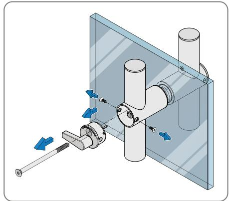
3. Insert the Lock Indicator thumb turn as shown below and secure it to the lock housing with the two lock housing screws.
