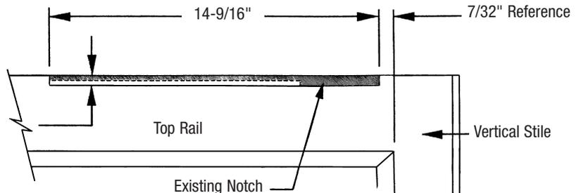
Mark Arm Clearance Slot as Shown Above.
