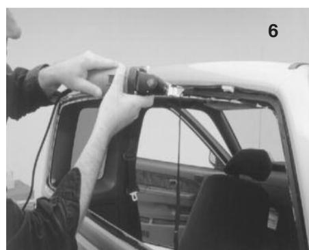
Using CRL Chisel Blade, trim down existing urethane bead all the way around opening. See photo 6.
