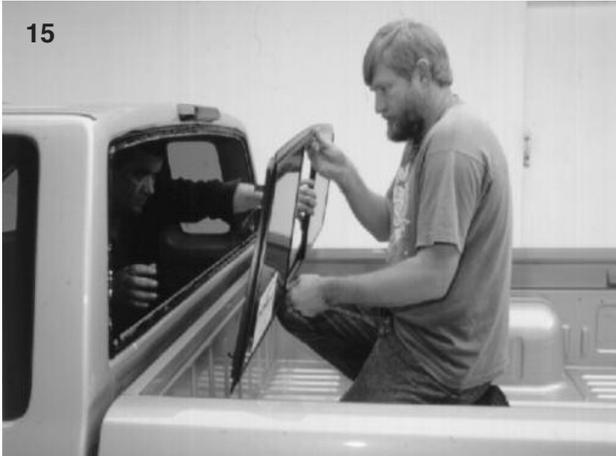
Carefully pick up the Tri-Vent and bring it to the cab opening. See photo 15.
