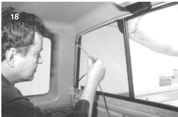
Reinstall black plastic trim piece around window opening on inside of cab. Hook inner leg over lip of pinchweld and press into position. Where trim piece goes over each bend-over tab, carefully notch trim for clearance if necessary. Install across the bottom, seating corner for proper alignment. See photo 20.
