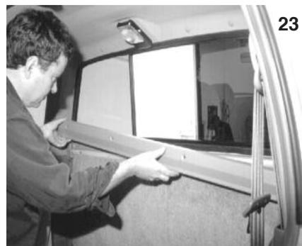
Reinstall screws, being careful not to over tighten. See photo 24.
