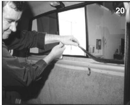
Across the top of the opening, cut off inner lip of trim piece where needed for clearance with upper slider track. See photo 21.
