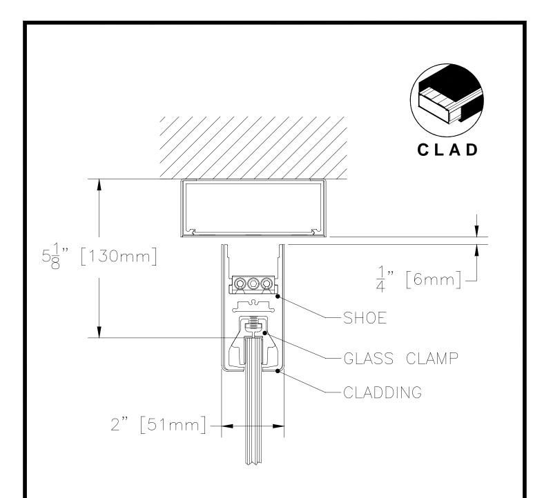
4" SQUARE DOOR RAIL CLAD WITH CLAD HEADER
