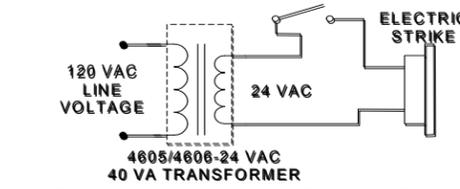
**TYPICAL ELECTRIC STRIKE WIRING DIAGRAM
