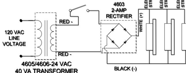
**TYPICAL ELECTRIC STRIKE WIRING DIAGRAM
