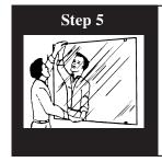
Mark the center of the mirror at the Bottom. Set the mirror in Bottom Clips aligning the centerline of the mirror with the centerline of the Bottom Hanger. Next lift the Top Clips on the Top Hanger and lay the mirror against the wall. Once the mirror is in place press the Top Clips downward over the edge of the mirror.
