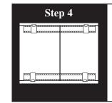
After the Bottom Hanger is installed measure up from the base of the Bottom Hanger Clips the height of the mirror less 1/2" (12.7 mm) and mark a horizontal line. Line up the centerline of the Top Hanger with the plumb vertical centerline on the wall and install the Top Hanger below the horizontal level line.
