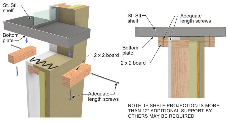
A. Drill and countersink 2" x 2" boards in the appropriate attachment area. Secure the 2 x 2 boards to both sides of the wall even with the bottom of the opening. Secure the shelf from the underside using screws of adequate length (not included).
