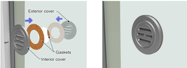
5. The Speak Hole Cover is packaged separately during shipping, inside the window package. Remove the screw, and separate the interior and exterior covers and gaskets. Insert the exterior cover and gasket on the glass cut out from the exterior side. Place the interior cover and gasket on the glass cutout from the interior side. Secure by fastening the screw through the interior cover and tighten.
