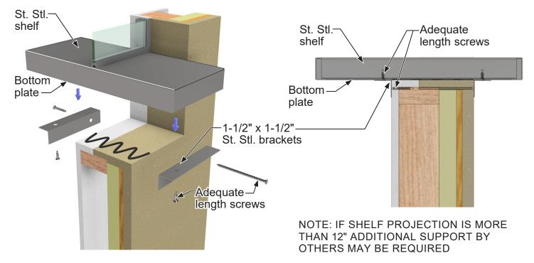
B. Drill and countersink 1-1/2" x 1-1/2" St. Stl. brackets in the appropriate attachment area. Secure the 1-1/2" x 1-1/2" St. Stl. brackets to both sides of the wall even with the bottom of the opening. Secure the shelf from the underside using screws of adequate length (not included).
