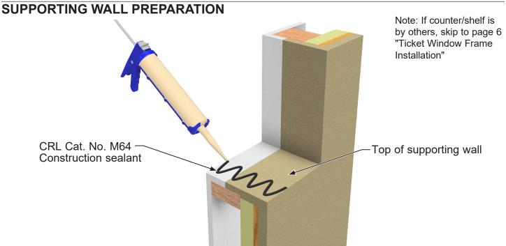
1. Apply **CRL Cat. No. M64** construction sealant between the shelf's bottom plate and the top of the supporting wall for additional strength.
