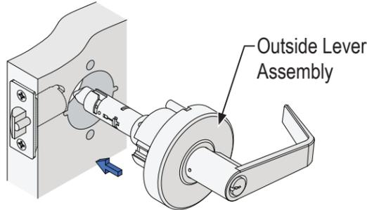
Install outside lever assembly on the door. Make sure tail of latch engages with retractor correctly as illustrated.
