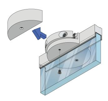
7. Remove the Interior Overhead Closer Adapter Cover.
