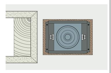
5. Grout the box in place using a Non-Shrinking or expanding grout.
