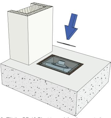
6. Tilt the BP-13 Pivot toward the doors exterior side, place the Finish Ring onto the spindle
