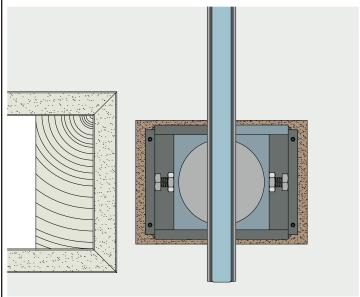
16. Adjust the gaps between the adjacent door/sidelite by adjusting the Pivot Screws, loosen the locking nuts prior to making adjustments. After making the adjustments secure the BP-13 Pivot by tightening the bolts against the box and tightening the nuts.
