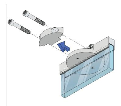
8. Remove the Spindle Clamp by removing the (2) 5/16-18 Socket Head Cap Screws.
