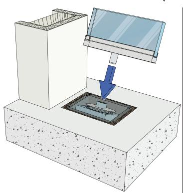
9. Install the door by inserting the bottom door rail pivot pin into the BP-13 spindle.
