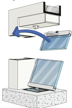
10. Tilt the door onto the overhead closer spindle and engage the spindle adapter.
