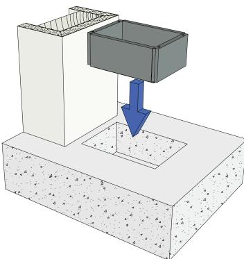
2. Place the BP-13 Pivot Box into the opening and shim the box flush with the finished floor.
