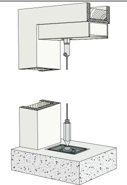
4. Use a Plumb Bob to align the BP-13 Pivot to the Concealed closer spindle above.
