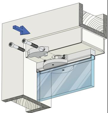
11. Re-install the spindle clamp with (2) 5/16-18 socket head cap screws.
