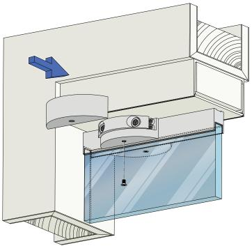
15. Re-install the Overhead Interior Closer Adapter Cover.
