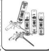
Screw the can onto the gun coupling, with valve upright, until it will go no further. Do not over tighten. Once attached, grip the can and the gun with both hands and shake well (15-20 times). Immediately pull the dispensing gun trigger to fill the gun with foam sealant. Adjust the larger metering screw to the required extrusion rate / bead size.
