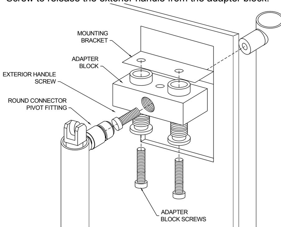
At the TOP Adapter Block, loosen up socket set screw and pull exterior handle away loose.
