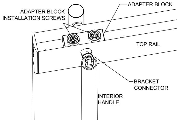
Install the Adapter Block into the Top Rail. Insert the handle fitting into the Adapter Block and tighten the setscrew.
