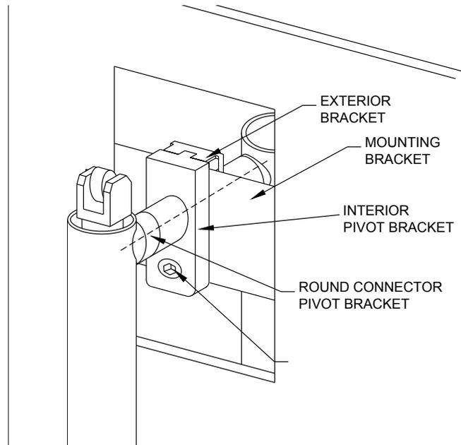
3. Remove threaded pin from bottom of horizontal handle and pull horizontal handle away from plywood. Use the **CRL Spanner Wrench** (part number MPH5W) to remove exterior horizontal handle retainer and rubber bushing.
