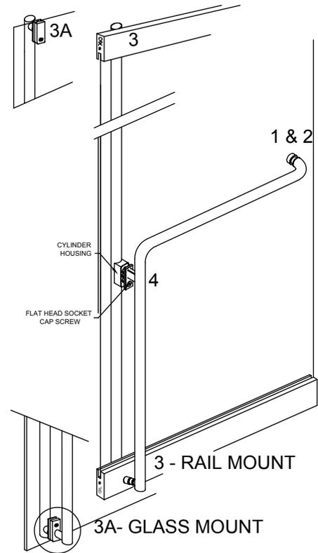
1. Push exterior retainer with rubber bushing through glass hole from interior side, into horizontal handle, and tighten with spanner wrench. ↓
