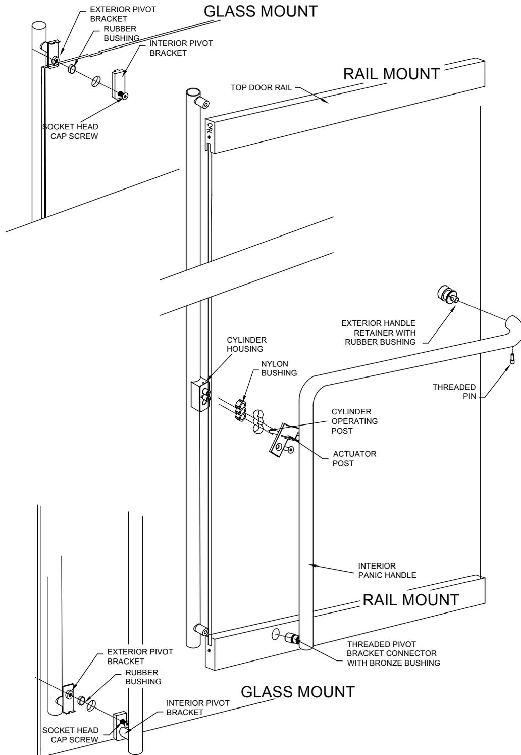
**Apply THREADLOCKER to all fasteners used to mount handle on doors.**
