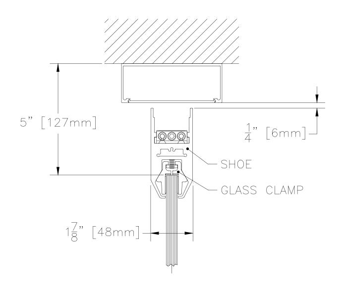
4" TAPERED DOOR RAIL UNCLAD WITH UNCLAD HEADER
