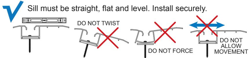
Do not overtighten fasteners. This can cause the sill to bow and/or distort and interfere with door operation. Clean cuttings from drill holes and any other debris from track.
