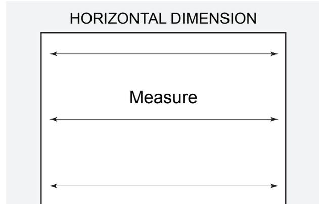
Measure side to side at top, middle and bottom to confirm proper width.
