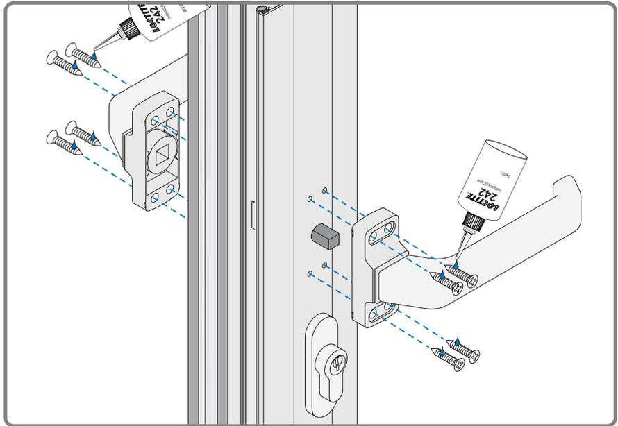
\*💧 Loctite® is recommended on all screw threads during final assembly.
