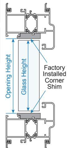
**NOTE:** Include Factory Installed Shim in calculations.
