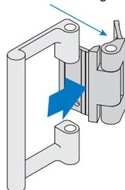
Insert 4-1/2" Hinge Pin with Knurled Side Up
