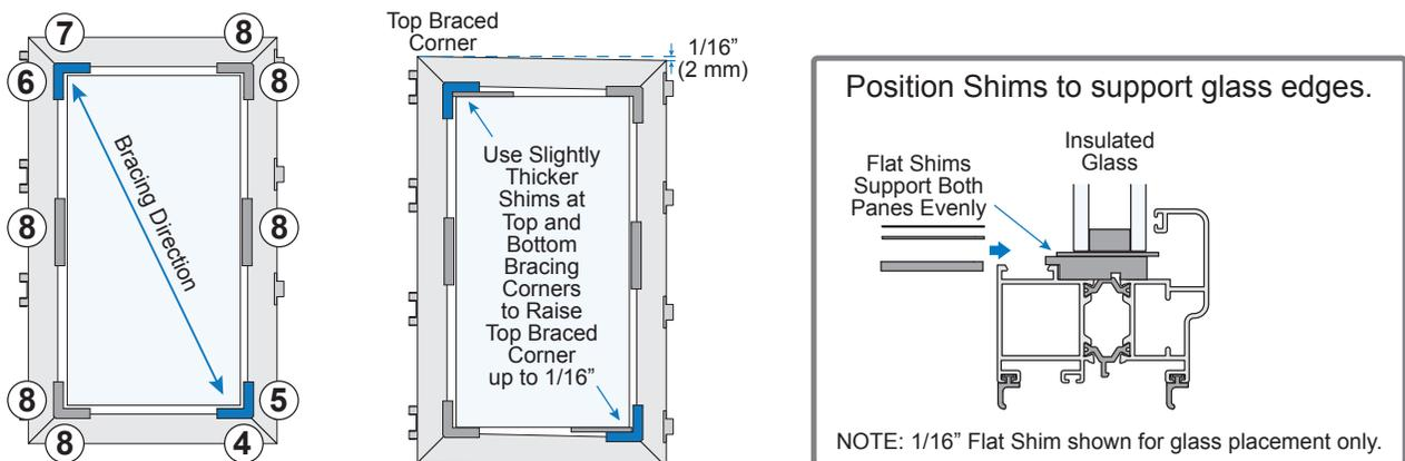
**NOTE:** When installed, the doors pull down slightly due to weight and the out of square doors become almost even. If there are any issues with door operation, shim thickness needs to be adjusted. Doors must be braced correctly for proper operation.
