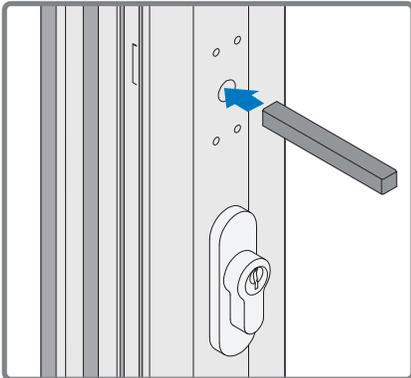
Install Handles on each side with included screws.
