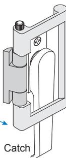
Fit Auxiliary Handle over Hinges when Installing Doors
