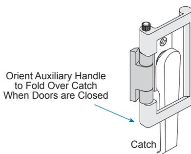
Orient Auxiliary Handle to Fold Over Catch When Doors are Closed
