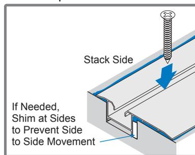
Slide Guide along Sill to test. Adjust screws to level track.
