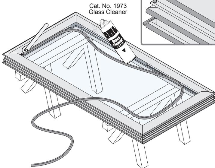
NOTE: Do not stretch gasket when installing. It should be cut approximately 1/8" (3 mm) longer and squashed in to allow for gasket shrinkage.
