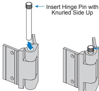
Insert Hinge Pin with Knurled Side Up
