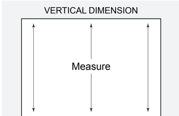
Measure top to bottom at left, center, and right to confirm proper height.
