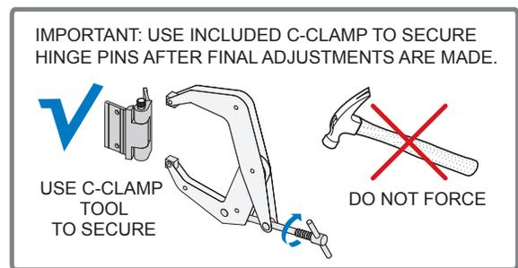
Use C-Clamp to push Hinge Pins securely into Hinges.
