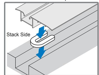
**NOTE:** Apply silicone under Sill for Exterior Installations.
