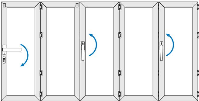
Lift Catch Handle away from plate to rotate up into unlocked position.
