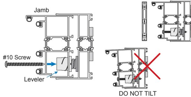
NOTE: Insert #10 fasteners appropriate for substrate into center of Levelers to secure. Do not overtighten fasteners.
