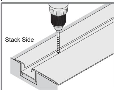
Remove Sill to drill holes and install anchors.
