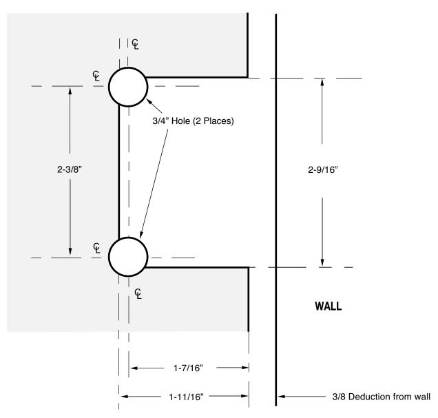
Note: Each hinge is located 8" on center from each end of the jamb
