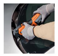
The heavier U-shaped blade is used for glass removal below hood level. Recommended speed: setting 3–4.
