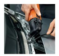
You can remove adhesive residue quickly, easily and effortlessly with the scraper blade. Recommended speed: setting 2-3.
