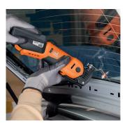
The type 143 cutter blade is equipped with an adjustable depth stop. This allows large windows to be cut out quickly and safely from the inside. Recommended speed: max. setting 3.
