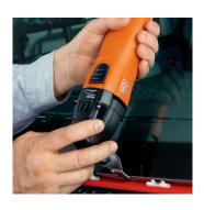
The U-shaped blades are used for glass removal below hood level. Recommended speed: setting 3-5.
