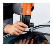
Encapsulated windshields and molded frames, including those with aluminum reinforcement, can be removed in one step using the L-shaped blade. Recommended speed: setting 3-4.
