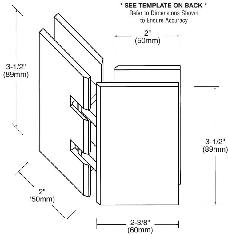
**(This hinge requires two different templates, one for the door and one for the mitered fixed panel).**
