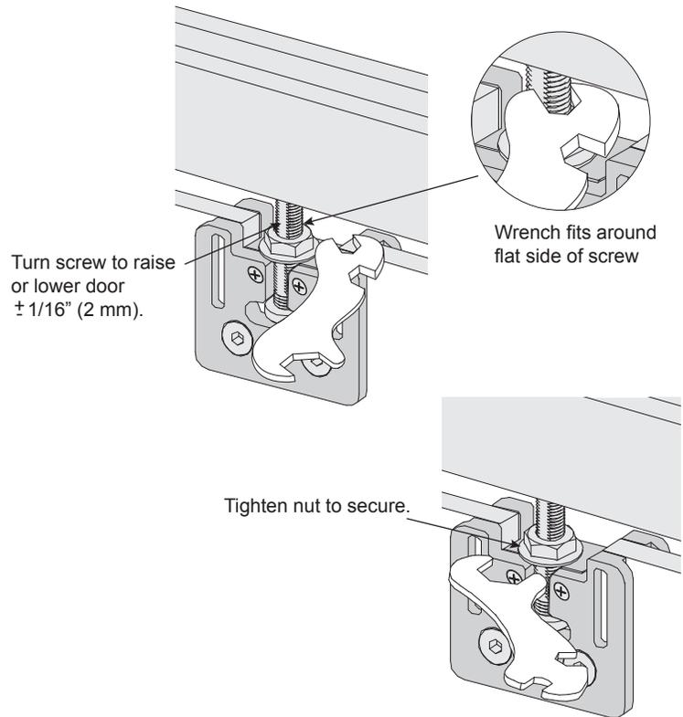
2. Adjust position of Dampeners and tighten screws to secure.
