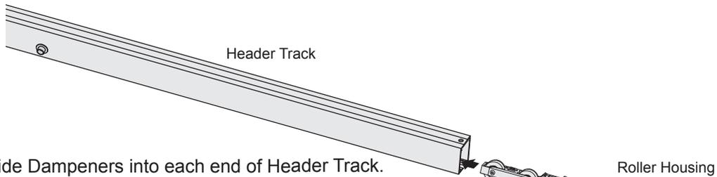
4. Slide Dampeners into each end of Header Track.
