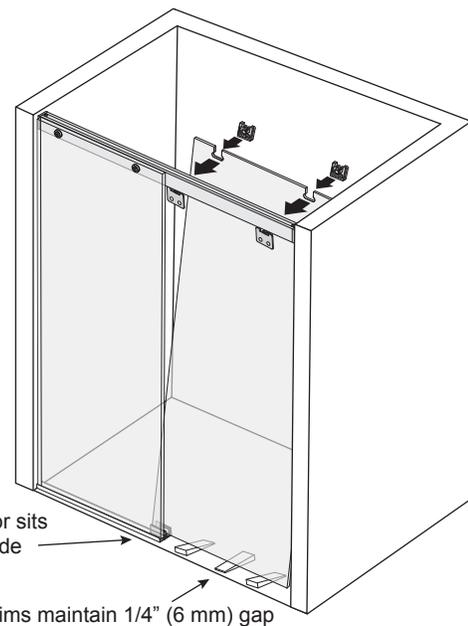
5. Fit each Interior Roller Bracket and secure.
