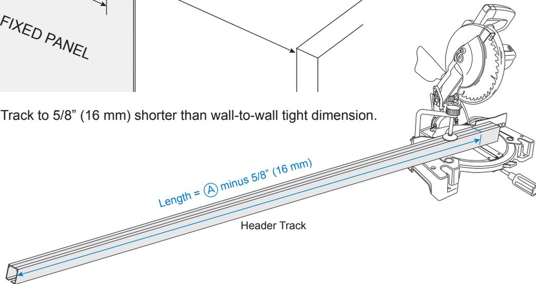
2. Drill 1/4" (6 mm) diameter hole 1/4" (6 mm) from end on top of Header Track at center on BOTH ends.
