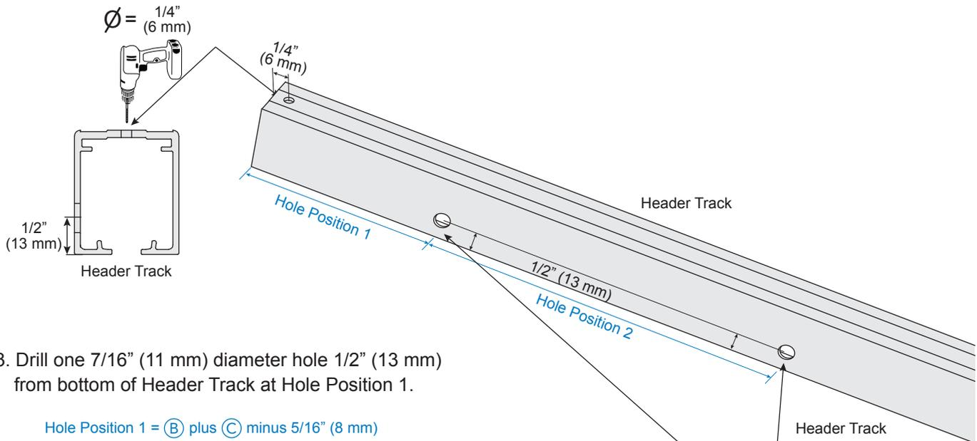
3. Drill one 7/16" (11 mm) diameter hole 1/2" (13 mm) from bottom of Header Track at Hole Position 1.
