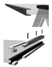
**Step 4:** Before tightening the screws lightly tap the top and bottom railsl snug to the end of the glass to eliminate any gaps. Check the alignment of the rails by measuring the overall distance between the top and bottom on the right and left side. Adjust until equal distance is achieved before proceeding to the next step.
