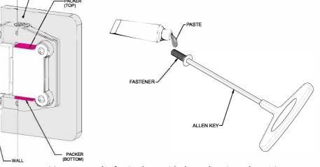
5. With correct gaps and packers in the correct positions, screw the fascia plates with the gaskets into place. Hinges are to be fitted straight and parallel. Using blocks + packers, place gate into position with extra 2mm higher at the latch end to allow for glass weight droop. Mark, drill and plug holes into the wall with secure fasteners
