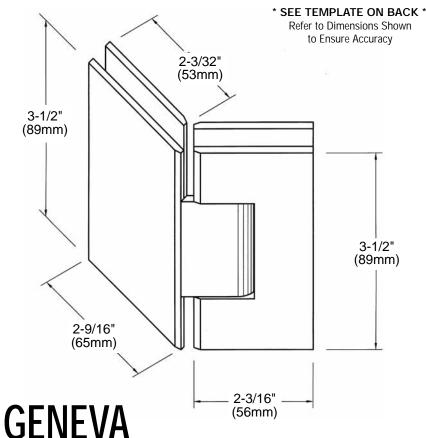
135° Glass-to-Glass Hinge Cat No. GEN345 (Adjustable) (This hinge requires two different templates, one for the door and one for the mitered fixed panel).
