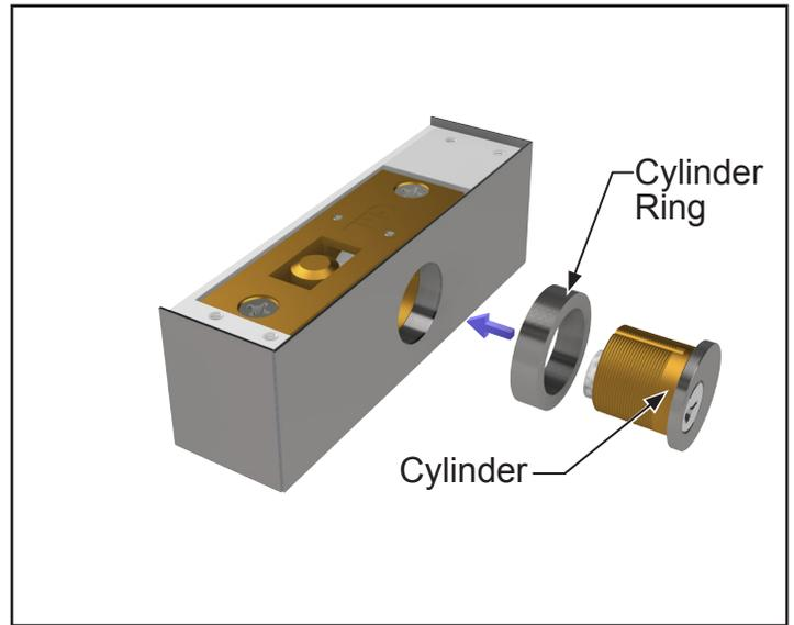
2. Install cylinder ring and cylinder (Cylinder lock **MUST** be in the horizontal position).
