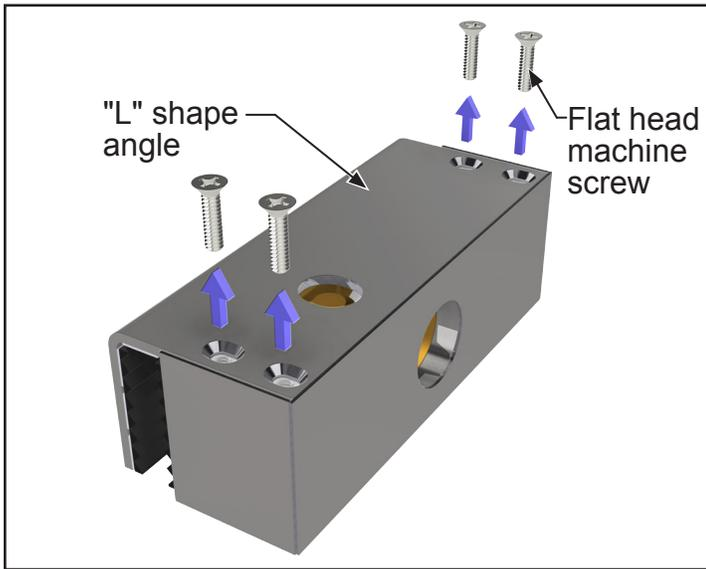
1. Remove (4) flat head machine screws and "L" shape angle.
