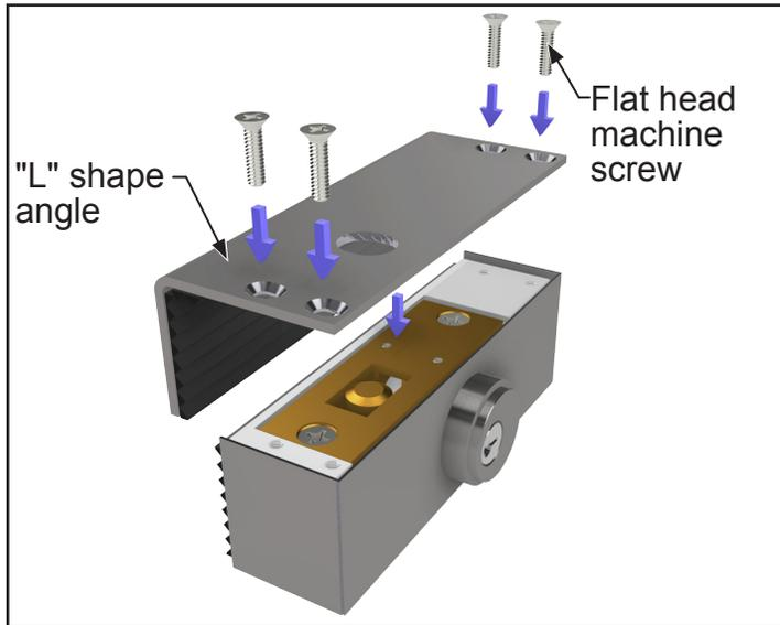
5. Re-install "L" shape angle and loosely secure with (4) flat head machine screws.
