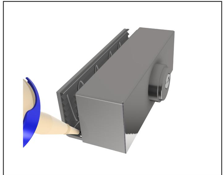
6. Apply **CRL 95CBL** silicone to lock body gaskets (Sides and Bottom).
