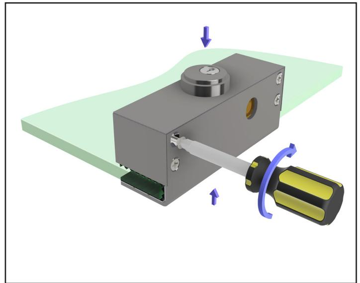
8. Compress the "L" shape angle to the glass panel and tighten (4) flat head machine screws.
