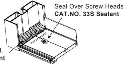
Sill to Subsill, End Dams, Screw Heads and Threshold to Door Frame Sealing.
